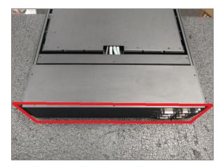
Step 2: Pull the drawer all the way out and release the locking mechanism to detach the drawer out of its bottom chassis, and please pull slowly and carefully to prevent the damage of falling drawer.
