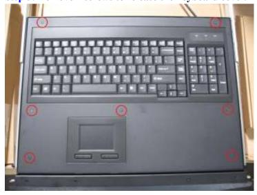
**Step 4.1:** Remove the 6 screws to release the keyboard
