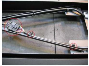
**Step 3:** Remove 7 screws to release the keyboard cover.
