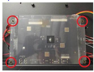
**Step 5:** Flip over the AD board and disconnect all the connected wires, and then replace with new AD board.
