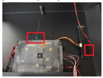
**Step 4:** Remove these 4 screws to release the AD board.
