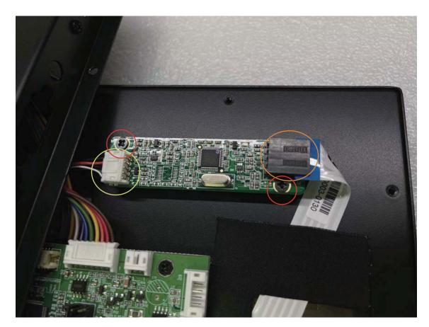
(4)Disconnect of USB cable (yellow circle), FFC(orange circle), unscrew and take the broken controller board off.
