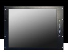
8U 19" 1280 x 1024, 250 nits rack mount LCD monitor AtoD Board (Model: DA005) OSD Control HDMI, VGA, CVBS-in(BNC)x2 CVBS-looping(BNC)x2, Audio (PIP) VESA Mounting & Built in Power Supply OSD on Front bezel right side
