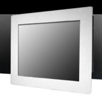
NEMA4x/IP65 Stainless Steel Panel Mount with Glass (Front Bezel 3mm), 17" LCD Monitor 1280 x 1024, 300 nits , Side OSD, including rear screw/Clamp/VESA Mount +PCAP Touch 10-points touch in Windows 7/10 with USB interface +JIMB-1900-2L / RAM 4GB ( 0C~70C ) / SSD 256GB ( 0C ~70C ) +I/O ( waterproof connectors ) : VGA x1, RS232 x1, Audio x1, LAN x2, USB x2 with 24VDC Power Input and power adapter for testing Excluded OS installation
