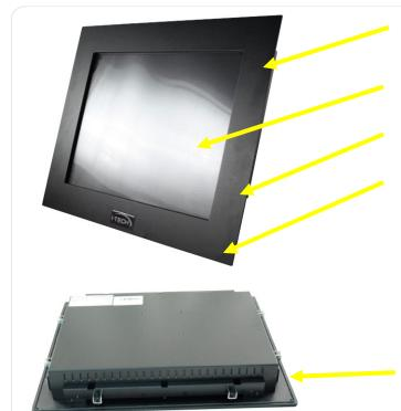
Metal 5mm Panel Mount for easy installation with stud mount and Clamps mount (Optional for Front AR Glass or Vandal Resistant glass)
