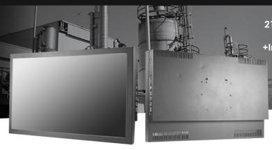
21.5" LCD monitor, 1920x1080, 300nits VGA Input, Side OSD with 5 Wire Resistive Touch Screen and USB Controller +Integrated DC 9-36V Input (Built-in). Terminal Block "+" and "-".
