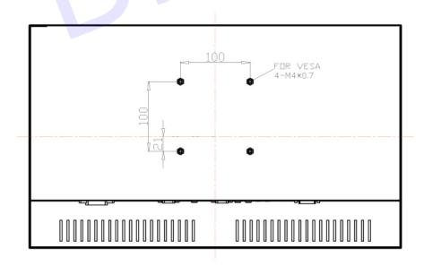
Drawing No.: ECHW2155D-FHD-PCT-V1-07062022-V1
