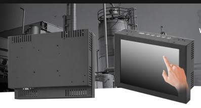
Wide Temp/Wide Viewing 10.4" LCD monitor, 1024x768, 1000 nits VGA+HDMI+ DVI Input, Side OSD, Wide Viewing angle, WV(178/178 MVA), Wide Temp (-30~70C) with 5 wire Resistive Touchscreen and USB controller
