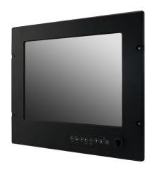
12.1" Marine Panel Mount LCD Display IP65, Rugged, 1024x768, 1000nits, 0-100% Dimming, wide Temp -15 ~ 55C and 24V DC-in with Isolation (Approval by Certificate) 9~36V DC Input Acceptable, 1x VGA, 1x DVI-D, 1x Composite 1x S-Video, 1x RS232 for Remote Control, w/ Resistive Touchscreen.
