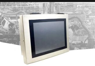
15" 450nits 1024x768 Fanless -20 to 60C Core i5-6200U2.3GHz Skylake Class 1 Division 2, ATEX Zone 2, and IECEx Certified 4GB Wide Temp. 128G SSD Wide Temp + Resistive Flat, NO OS
