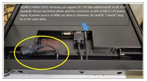
ELDW117HDFe can support both AC or DC 12V (No additional DC to DC PS is needed). Please see attached photo and the connector on left of DVI is 12V power input.
