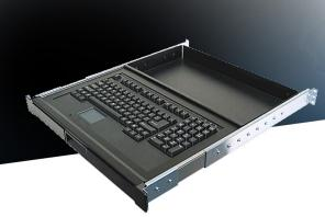
1U Rackmount 104 key full size keyboard with numeric pad, Centered two button touchpad, 8.5" deep storage space behind keyboard. Slides adjustable for 22.75" to 31.5" rack mounting depth, 19"(W) x 1.75"(H) x 20.0"(D)
