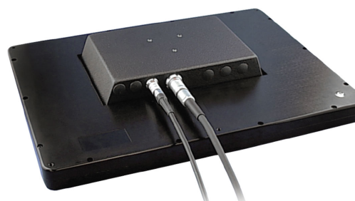
Standard cable length is 10 ft; inline amplifiers recommended for longer cable.
