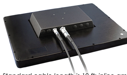
Standard cable length is 10 ft; inline amplifiers recommended for longer cable.
