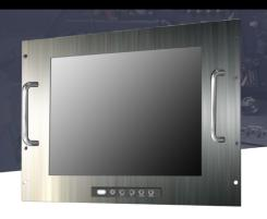
19" Industrial Panel / 1280x1024 / 1000nits (Backlight Module Modified) with Resistive Touch I/O (all connectors are waterproof connectors / 6ft long): VGA, DVI, USB (for Touch use) and 12VDC with external 100-240VAC Power Adapter
