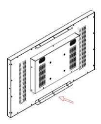
Step 2 fix the L-bracket on the monitor
