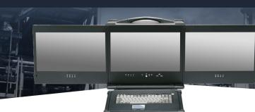
Rugged portable enclosure with rubber corners, 3x17.3" LCD (1920x1080 Resolution/each display) 3xDP connectors with Intel Core i7, Pro WS W680-ACE, Complimentary Carrying Bag with wheels
