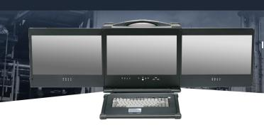
Aluminum alloy portable server enclosure with rubber corners 3x 17.3" LCD (1920x1080 Resolution), DP Connectors with Single Intel Xeon Gold 6312U, Complimentary Carrying Bag with wheels
