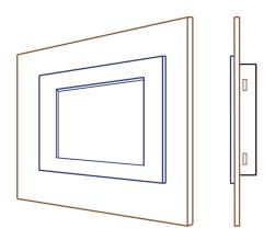
4-2. At the back side of the mounting wall, insert the mounting kits into the slide hole at the side bracket on the panel.4-3. Put the screw on the mounting kits and screw it tightly.
