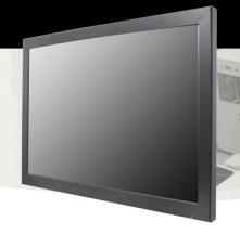
Front Water and dust Proof IP65/NEMA 4 with IP65 Solid Back Housing except I/O. 65" Panel / 1920x1080 / 450nits, Chassis Design / Wall mount, IR Touch, Speakers, I/O: VGA, DVI, HDMI, USB (for Touch use) and 100-240VAC power cord
