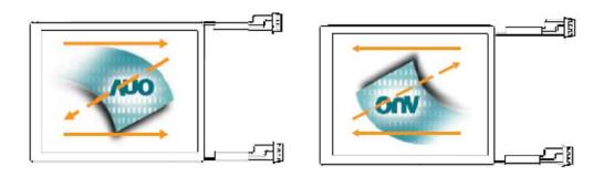
Fig. 1 Normal scan (Pin4, REV = Low or NC)
