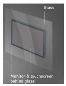
Suntronic Touch<sup>™</sup> can be applied directly to a window or a glass sheet with a rear projection screen
