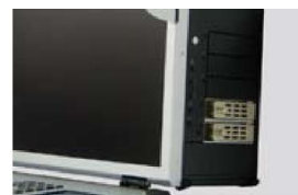
7x 3.5" removable HDD trays for data storage
