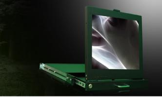
The DRP Series is an high performance 1U LCD display drawer sporting 15", 17", and 19" LCD Monitors. These monitors have high contrast ratios and wide viewing angles with resolutions at SXGA (1280X1024) for the 17" & 19" monitors, and XGA (1024x768) for the 15" monitors.
